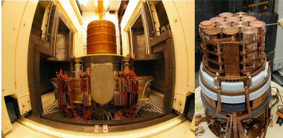
Active muon veto ( $>98\%$  coverage) on mobile shield
