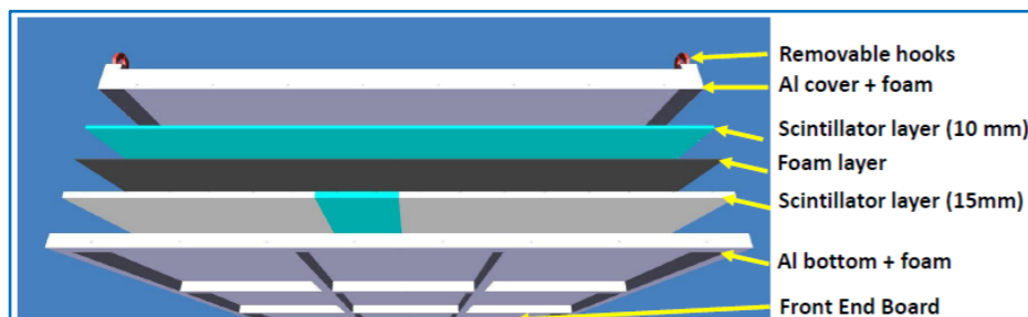
Cosmic Ray Tagger capable of measuring the position and time of entering charged tracks to the TPC volume.
