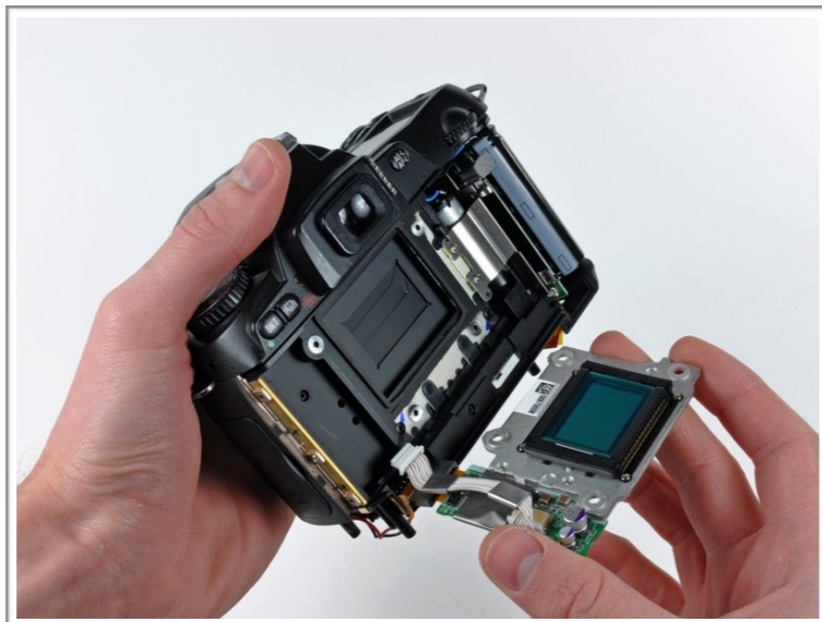
Image sensors ~ 10-20 \mu\text{m} thick CCD
