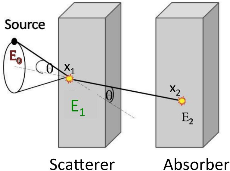
Compton kinematics to reconstruct the cone shell where the source must be contained
