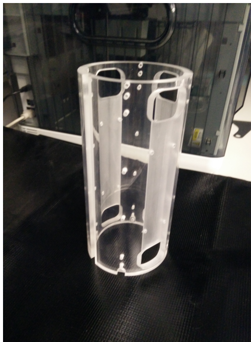
FIG. 7. The DArT external acrylic cylinder
