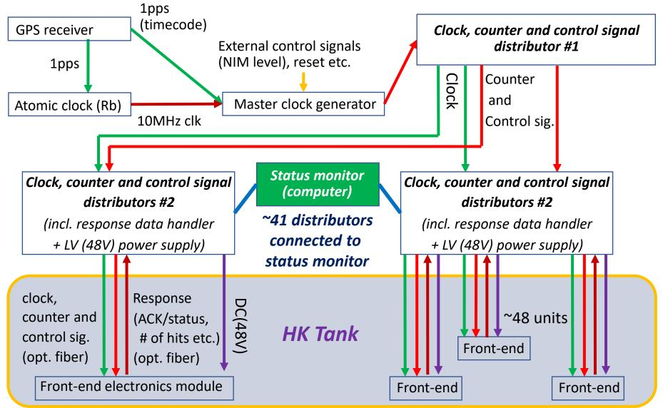
48 front-end elec. modules are connected to 1 distributor
