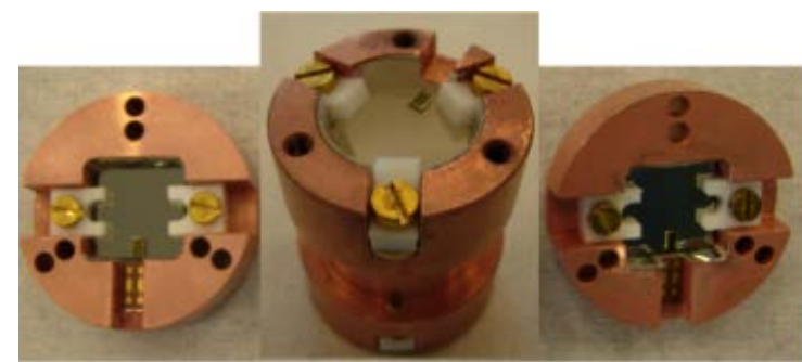
Scintillating Bolometer ZnMoO4 and its 2 light detectors LUMINEU @ LSM, France
