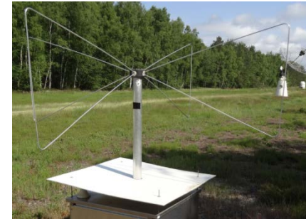
Butterfly Antenna, 2.2 x 1.5 m Codalema @ Nancay - France
