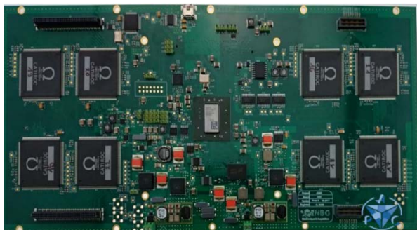
128 small PMTs RO Board – 8 CATIROC chips
