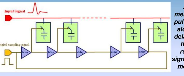
An analog memory: a write pulse is running along a folded delay line (DLL). It drives the can be only a recording of subset of the signal into analog whole channel memory cells.
