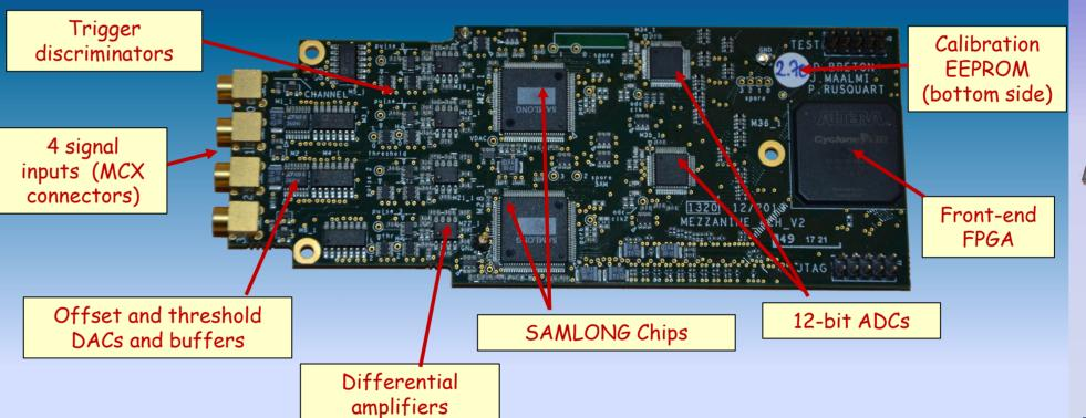
**Application Examples** These acquisition systems are used in test benches or experiences in a multitude of labs,
