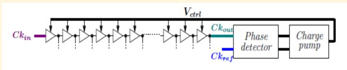
Principle of the single 64-cell DLL driving the 16 channels. It ensures a constant width to the write pulse even after trigger.
