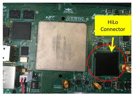
d. Plug the DDR4 memory module into the HiLo connector.
