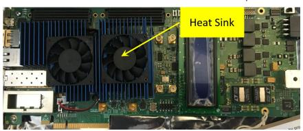
b. Remove the heat sink from the board by squeezing and pushing out the two pins from the back of the board.
