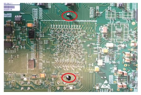
c. Locate the HiLo connector that was previously hidden by the heat sink
