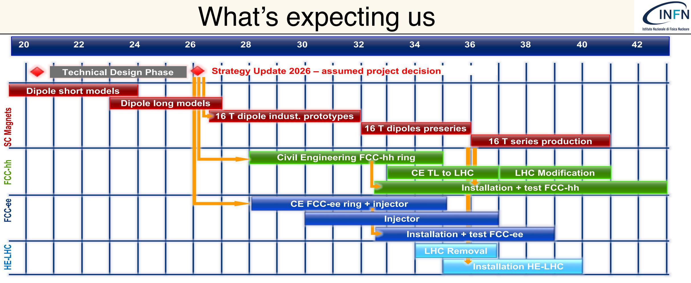
HL-LHC will work until 2037. What after? Main goals: Extend HL-LHC reach in pp and PbPb, probe new physics at high mass, diHiggs HE-LHC: intermediate infrastructure between HL-LHC and FCC with a center of mass energy of 27TeV Using the same tunnel of HL-LHC, but FCC class magnets of I6T
