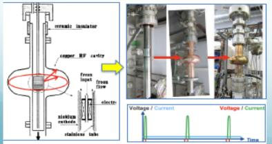
SRF cavity fabrication for high-gradient (N doping well stablished) and high-Q (N infusion, low-T baking to be understood)
