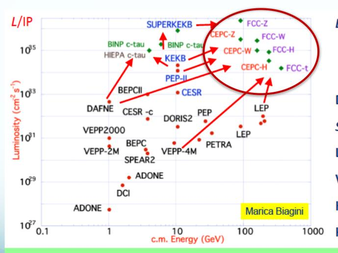
**B-factories:** KEKB & PEP-II: double-ring lepton colliders, high beam currents, top-up injection DAFNE: crab waist, double ring Super B-factories, S-KEKB: low  $\beta_v^*$ LEP: high energy, SR effects VEPP-4M, LEP: precision E calibration KEKB: e<sup>+</sup> source HERA, LEP, RHIC: spin gymnastics
