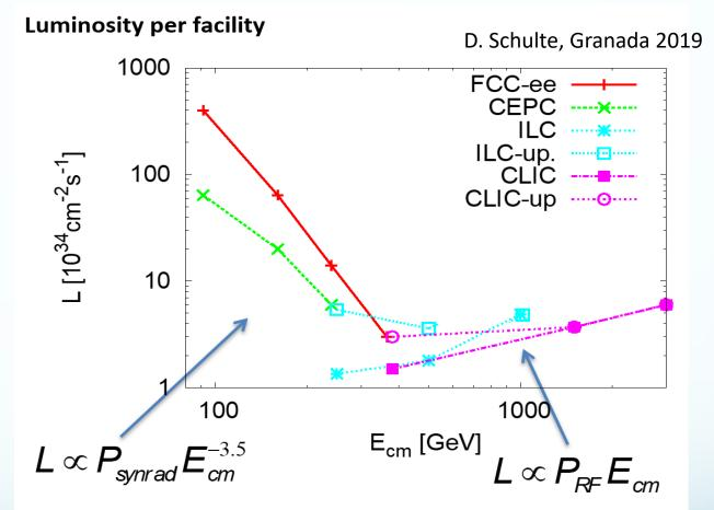
**Note: The typical higgs factory energies are close to the cross over in luminosity** Linear collider have polarised beams (80% e<sup>-</sup>, ILC also 30% e<sup>+</sup>) and beamstrahlung
