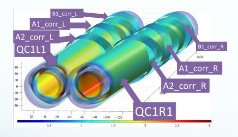
Final quadrupole pair near IP; canted-cosine-theta concept; with orbit corrector & skew quadrupole ; to be built with Nb-Ti or HTS wires • 2D field cross talk of QD0 two apertures near the IP side.
