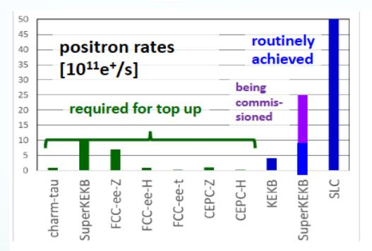
Routinely achieved positron rates: SLC, 1 bunch/pulse, 65 nC, 120 Hz, 5x10<sup>12</sup> e<sup>+</sup>/s KEKB, 2 bunches/pulse 2x0.6 nC, 50 Hz, 4x10<sup>11</sup> e<sup>+</sup>/s Under commissioning:
