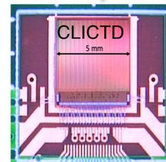
Modified HR-CMOS depletion (6V) with faster and higher rate readout capabilities
