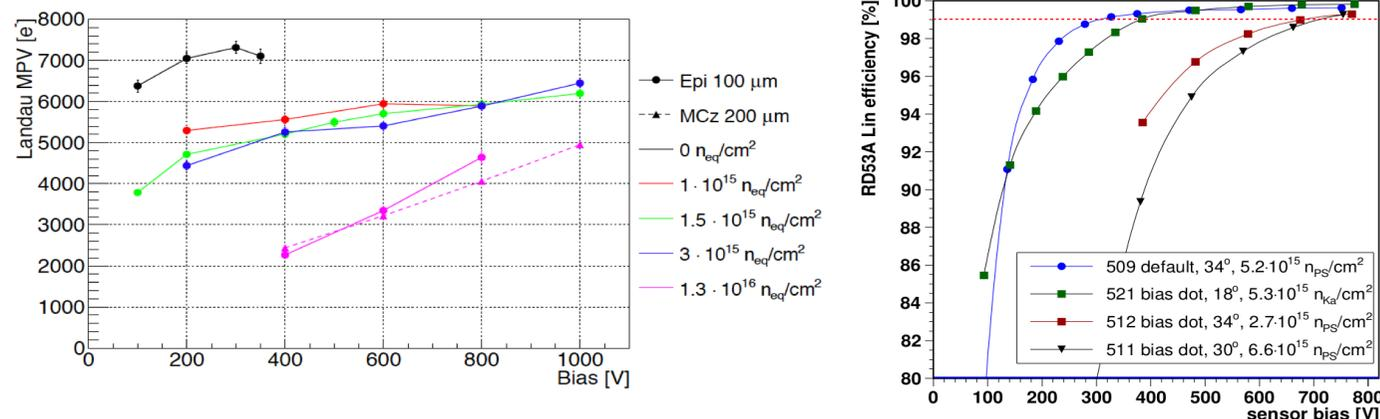
3D pixel sensors ongoing tests with RD53 chip: 1<sup>st</sup> layer in CMS<sup>1)</sup> should sustain at least  $\frac{1}{2}$  of 3000 fb<sup>-1</sup> with full efficiency at 150
