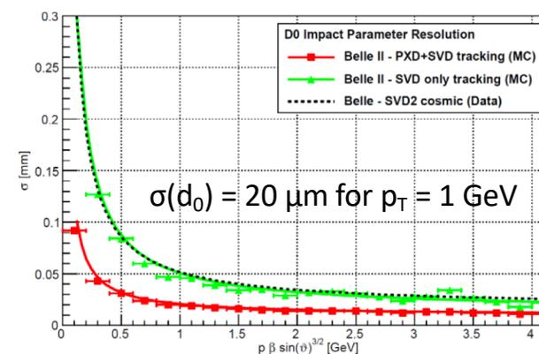
1) SVD is  $\approx 1\text{m}^2$ , 4 double side stereo layers at 3.9, 8, 10.4, 13.5 cm,
