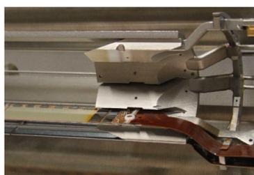
3D-printed support cooling blocks
