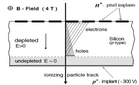
Charge sharing depends on diffusion<sup>1)</sup> in sensitive element,  $S/N$ <sup>2)</sup>, incident angle and B-field, Resolution<sup>3)</sup> optimization is a compromise in layer thickness, pitch and configuration parameters<sup>4)</sup>
