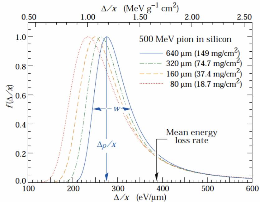
In Silicon  $dE/dx = 3.88 \text{ MeV}/\text{cm}$  and average e-h pair pair energy is 36 eV/
