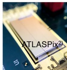
Modified HV-CMOS depletion (< 100 V) with faster and higher rate readout capabilities
