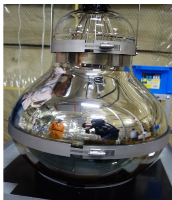
FIG. 106. Picture of the support bands attached to the B&L PMT.
