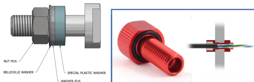
FIG. 140. On the left, a sketch of the dummy penetrator used for the hydrostatic pressure test at Resinex (Italy). On the right, a commercial penetrator. A glue could fix the Ethernet cable with the penetrator.
