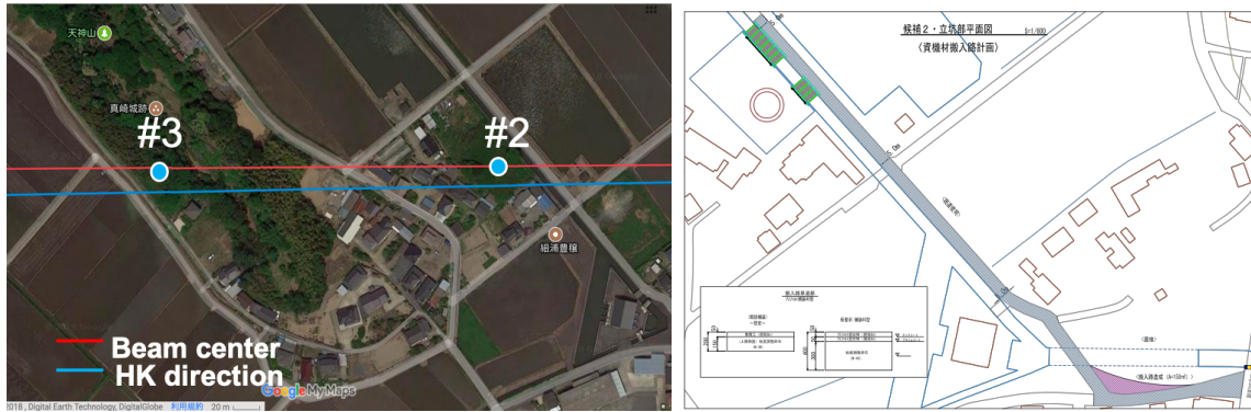
FIG. 66. Map around candidate #2 and #3. Red and blue lines show the direction of beam center and direction toward Hyper-Kamiokande (Tochibora site), respectively. Circle indicate the size of 11 m diameter pit although the position is not precisely fixed. Right-hand figure shows the extension of access road required to reach candidate # 2 (provided from construction consulting company).
