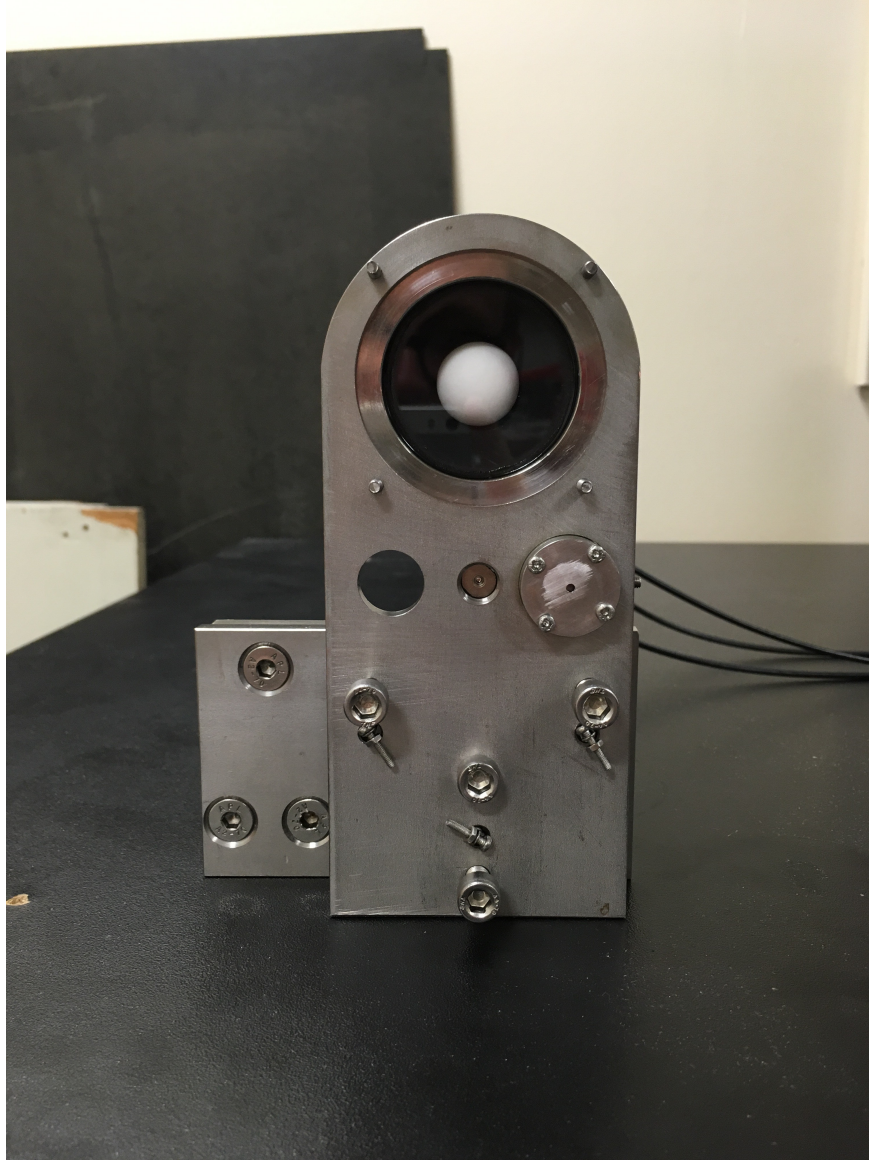
FIG. 149. Photograph of the light injector deployed in Super-K in 2018. The system contains a bare fibre (centre), diffuser (top) and collimator (right).
