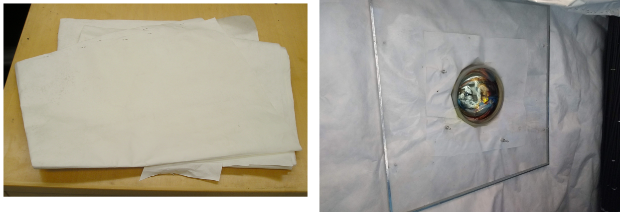
FIG. 117. Left: A piece of Tyvek sheet. Right: An OD photosensor mounted inside Super-K.
