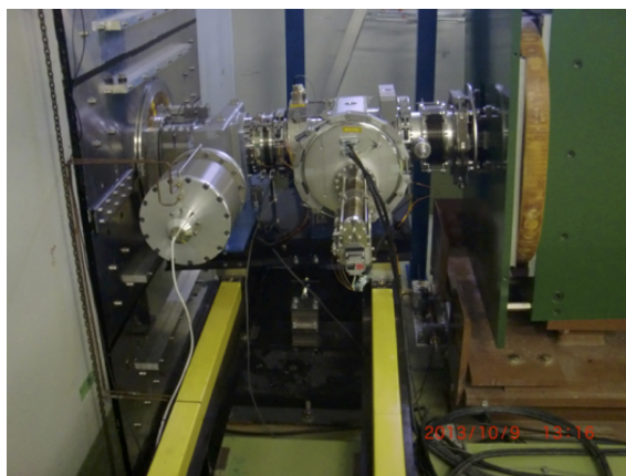
FIG. 5. The most downstream part of the final focusing section. The Target Station sits behind the wall on the left.
