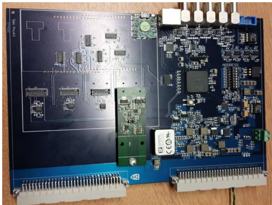
FIG. 150. Photograph of the LED driver system with mother board and daughter board that was deployed in Super-K in 2018.
