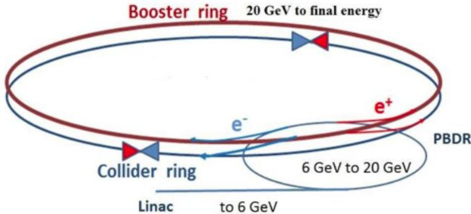
First-phase machine in the 100-km tunnel built to host eventually FCC-hh
