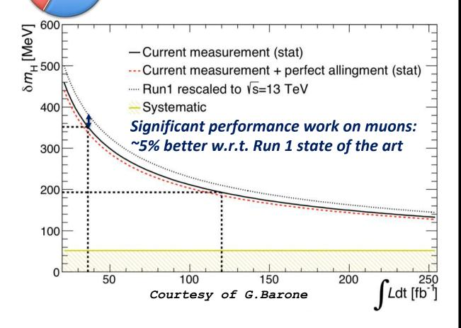
Key to precise Higgs boson mass measurement is the calibration of the ATLAS detector
