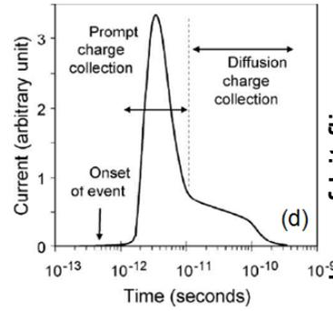
Current pulse caused by the passage of the energetic particle
