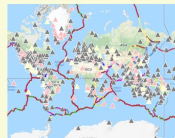
Real-time seismic stations currently received at INGV-ONT, this represents the backbone of data on which a global EEWS could be implemented.
