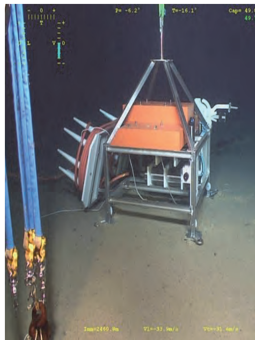
View of the Instrumented Interface Module (IIM) that is hosting a CTD sensor, an oxygen sensor, a turbidity sensor, a currentmeter (ADCP) (Credit: ANTARES)
