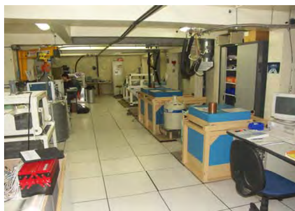
Gamma spectrometers protected by lead shielding at Underground Laboratory of Modane (Credit: LSM)
