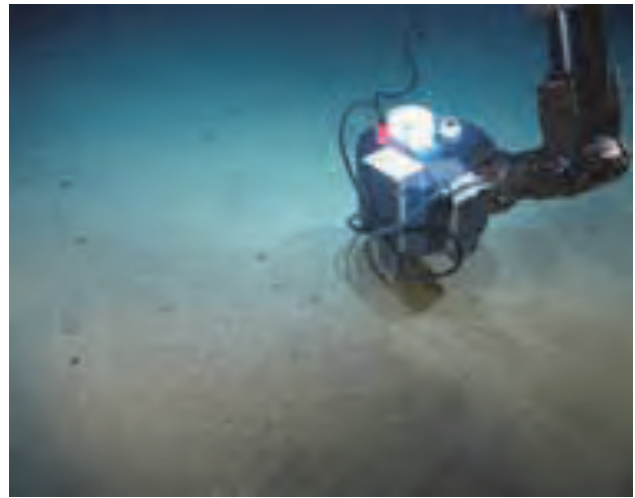
Seismometer connected to the ANTARES secondary junction box (Credit: ANTARES )
