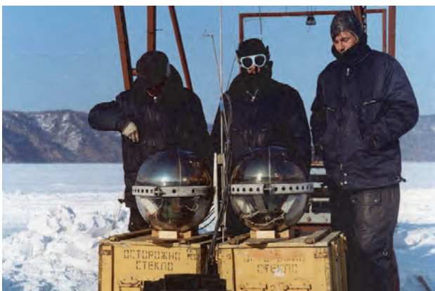
The optical modules of the Baikal Neutrino Telescope. The main part of an optical module is a large (37 cm diameter) high sensitive QUASAR photo-tube. (Credit: the Baikal Project).
