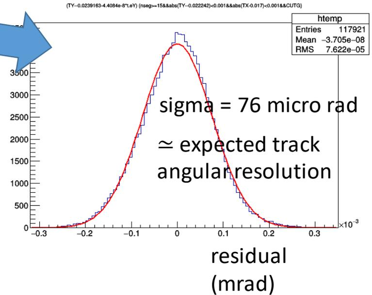
The “right-shoulder up” feature is consistent with a “diverging beam”.
