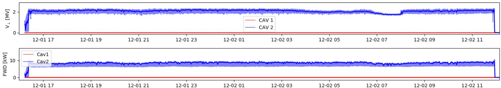
Note: After many hours of stable operation, we observed big thermal load and lost RF conditions, the trigger of such events is not fully understood
