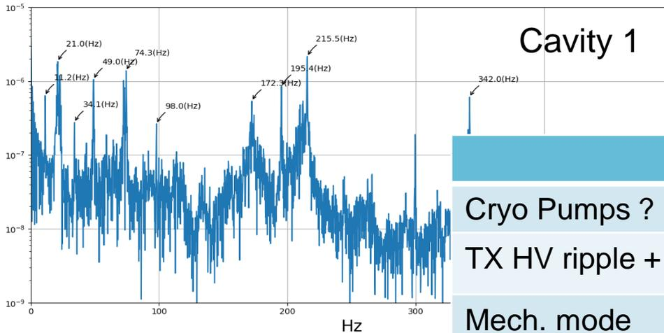
Due to small amplitude of detuning from microphonics, non-issue
