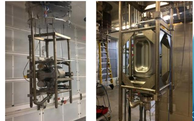
\* Voltage limit for SPS-DQW with HOMs due to inadequate BCP of HOMs
