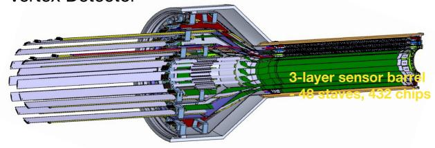
Service cone: signal, power, cooling and mechanical support
