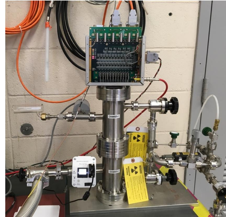
$^3\text{He}$  polarimeter test setup to measure null signal asymmetry.
