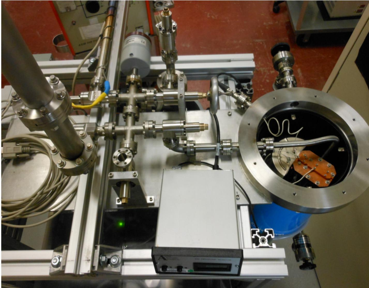
$^3\text{He}$  cyro-purification and storage system was built from a modified cryo-pump. Pumps everything except helium!
