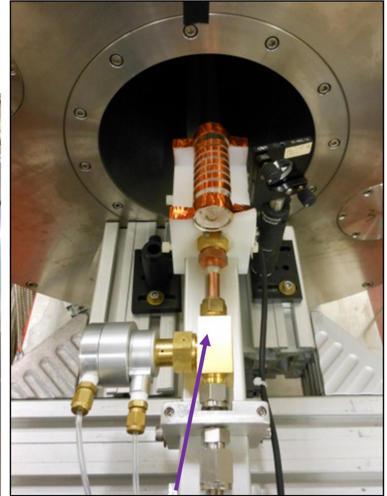
Non-magnetic brass pneumatic remotely controlled Isolation Valve
