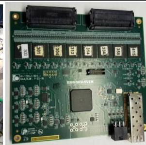
sPHENIX SAMPA + FELIX DAQ chain reading out EIC GEM detectors
