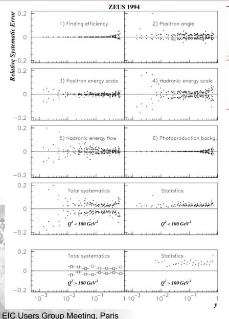
The systematic uncertainties are determined by changing something (e.g. calorimeter energy scale) within its uncertainties and determining the cross-section again.
