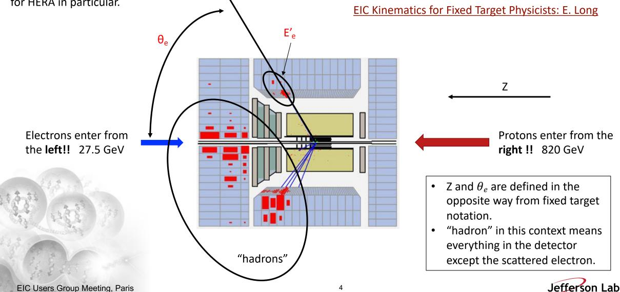
There is an important kinematical concept  $\sum_n (E - pz)$  where n is over all particles: E-p<sub>z</sub> for short. The initial (before collision)  $E-p_z = 2E_e$ , because  $E_p = p_{pz_r}$  and  $E_e = -p_{ez}$  (remember the direction of Z!)
