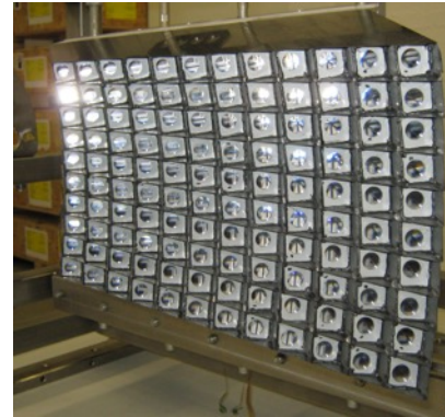
Barrel EMC alveoles and rear inserts
