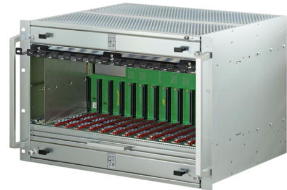
MicroTCA crate with CMS-style backplane
