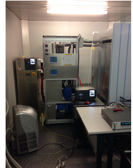
Custom cooling system at IPNL, can cool 2 sectors at -35
