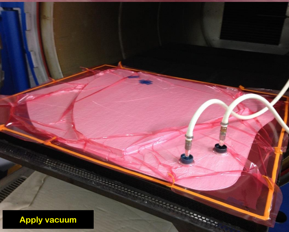
Autoclave 1 bar vacuum + 1 bar overpressure, 250C for 24 heures
