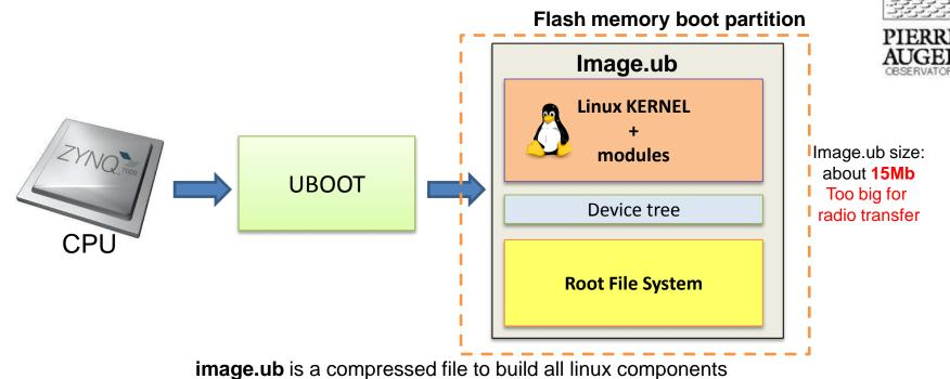
At system startup UBOOT decompress image.ub into the ram and lunch the kernel
