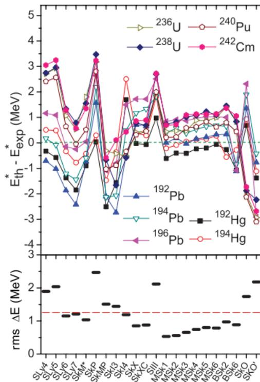
FIG. 5. (Color online) Residuals  $\Delta E = E_{\text{th}}^* - E_{\text{exp}}^*$  (top) and rms deviations from experiment (bottom) for various Skyrme EDFs. Additional references for the Skyrme forces: SLy5-SLy7 [88], SkMP [126], SkX-SkXC [127], SIII [128], MSk1-MSk6 [129], BSk2 [87],
