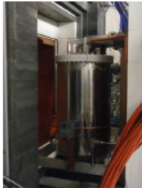
XENON100 Total Xe: 162 kg Target: 62 kg Fiducial: 34/48 kg Limit: \sim 10^{-45}
