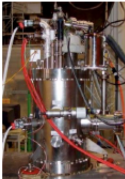
XENON10 Total Xe: 25 kg Target: 14 kg Fiducial: 5.4 kg Limit: \sim 10^{-43}
