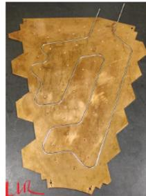
Cooling tests (optimization of Cu & tube thermal contact)
