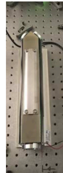
IR mode cleaner assembled and locked
