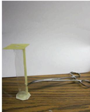
Figure 4: Clamp used to support the gluing of the endcaps.
