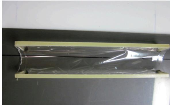
Figure 2: Placement of the tube after cut of the rest of the Mylar.
