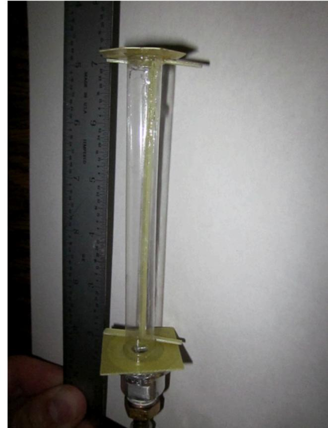
Figure 5: Test-tube with 8 Torr overpressure
