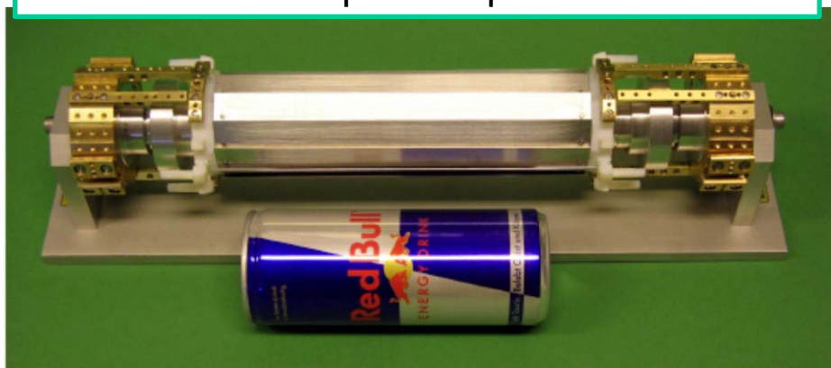
Mechanical mockup of the pixel detector
