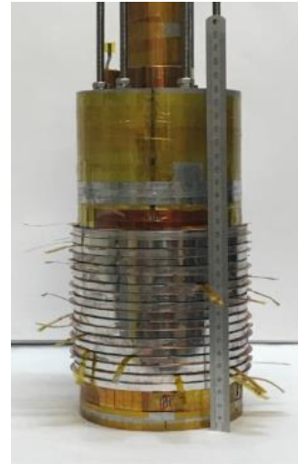
The Nougat solenoid (32.5 T) @ LCNMI Grenoble
