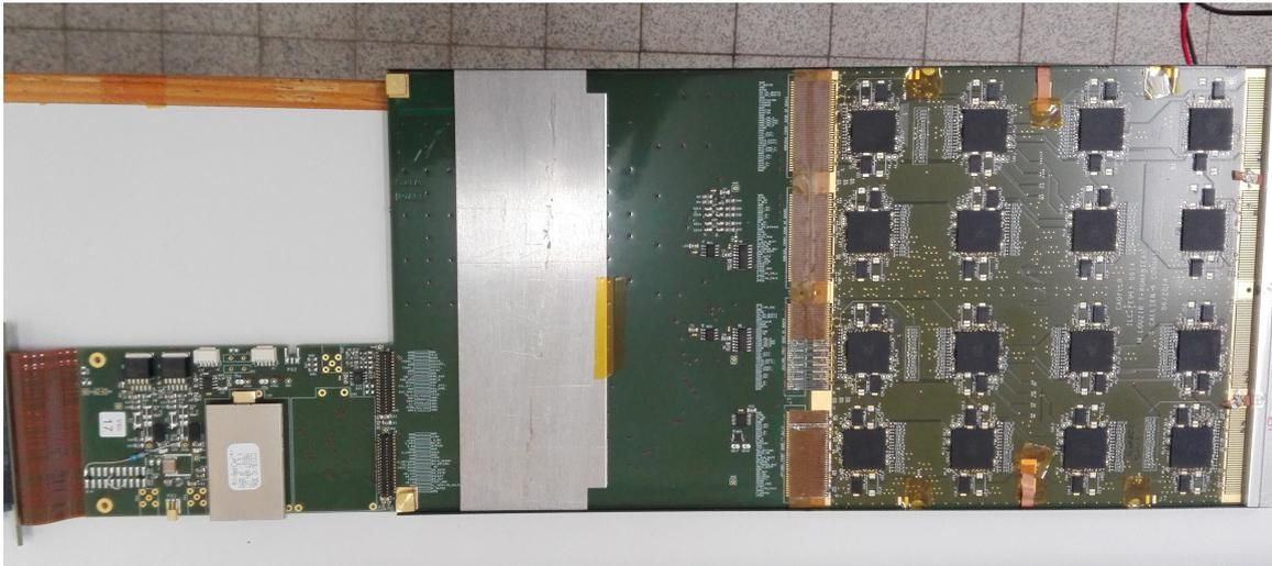
**Figure 3.** Open single SLAB with FEV11 ASU, 16 SKIROC 2 and the interface card visibles.
