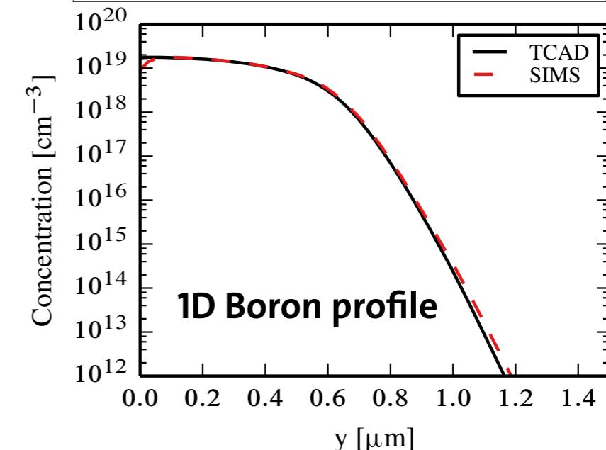
Simulation has to be calibrated with SIMS or other measurement on test structures for the same process
