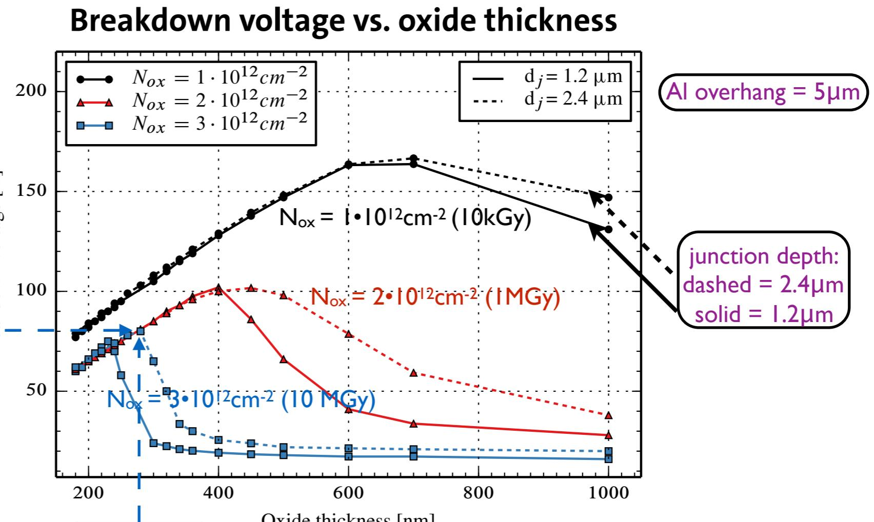
Optimum thickness: breakdown at edge of implant and edge of metal simultaneously
