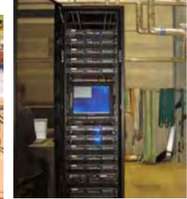
12-FEM board stack-up before burn-in phase
