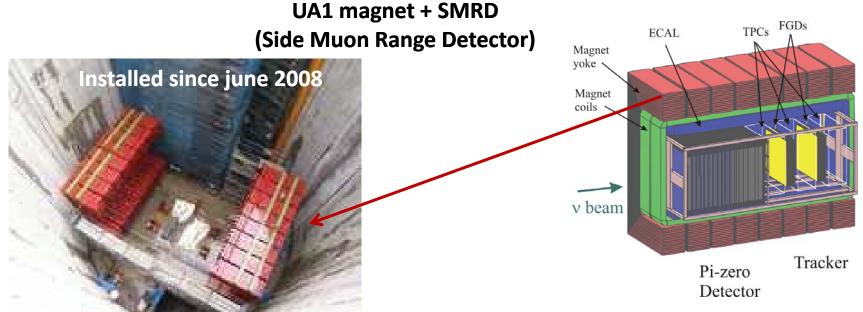
**8+8 C-shape elements** constituted of iron blocks interleaved by 17mm air gaps.
