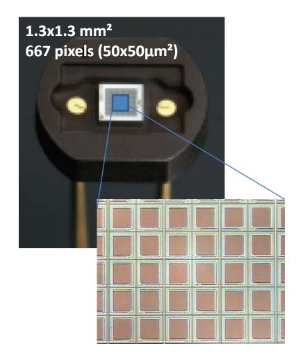
**60 000** MPPCs have been produced for the T2K experiment, used in several sub detectors: **INGRID, POD, SMRD, FGD**
