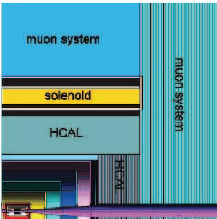
Figure 1.1: Illustration of a quadrant of SiD.
