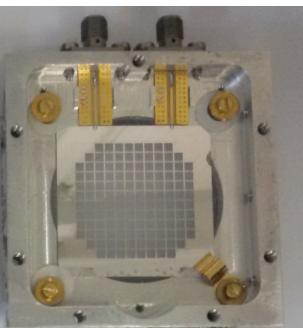
**LEKID Array for KISS Interferometer (300pix)**
