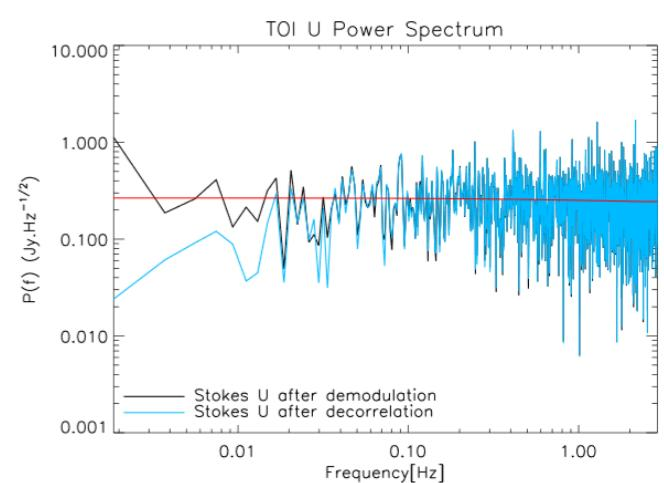
Flat noise spectrum thanks to the fast rotating half-plate (polarisation modulated at 12 Hz)
