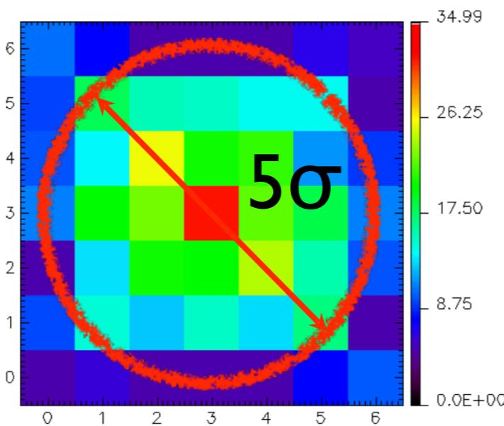
the surface of the silicon wafer impacted by a typical 200 MeV CR never exceeds a square of about **6x6 detectors** (about **1.4 cm<sup>2</sup>**).
