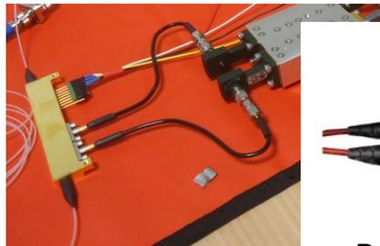
**DC-20 GHz Commercial MZM. Non-Integrated LiNbO<sub>3</sub> technology from Thorlabs**
