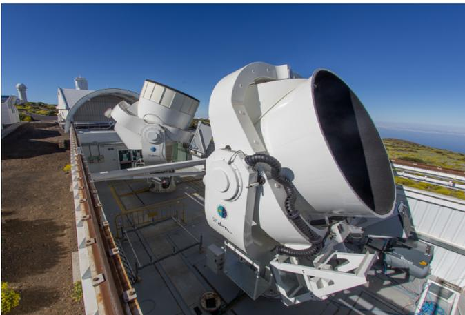
**KISS** : Low-resolution ( $\Delta\nu = 1-3$  GHz) Martin-Puplett interferometer (MPI) coupled to a **KID** based camera (80-280 GHz). Visitor instrument mounted at QT-1 telescope (Teide Observatory, Tenerife).
