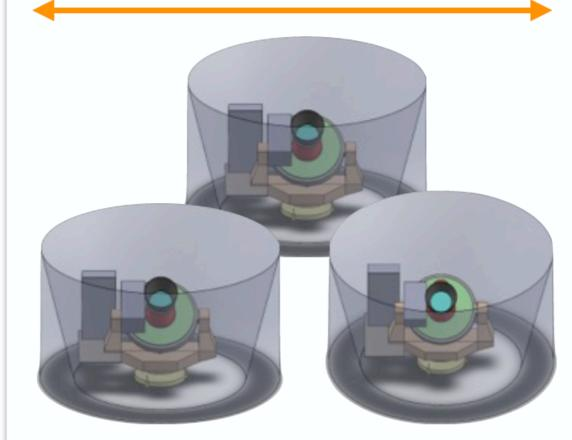
Three 42 cm diameter refractors, baseline dichroic pixels: 30/40 | 90/150 | 90/150 | 220/270 GHz
