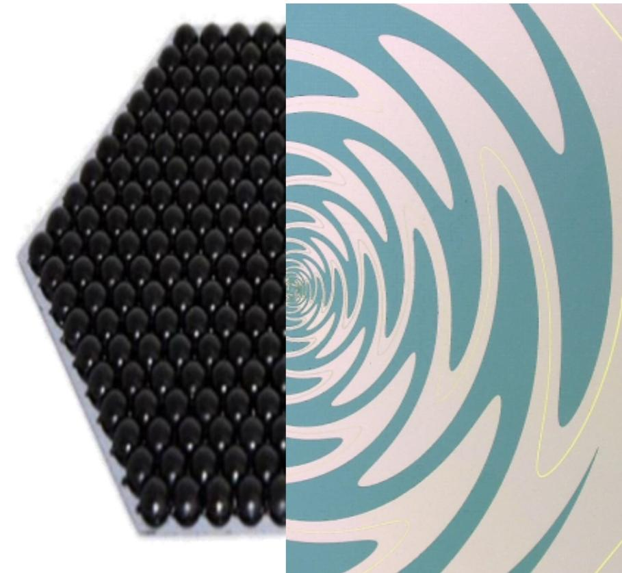
**Anti-reflection coated silicon lenslets coupled to sinuous detectors (Berkeley)**
