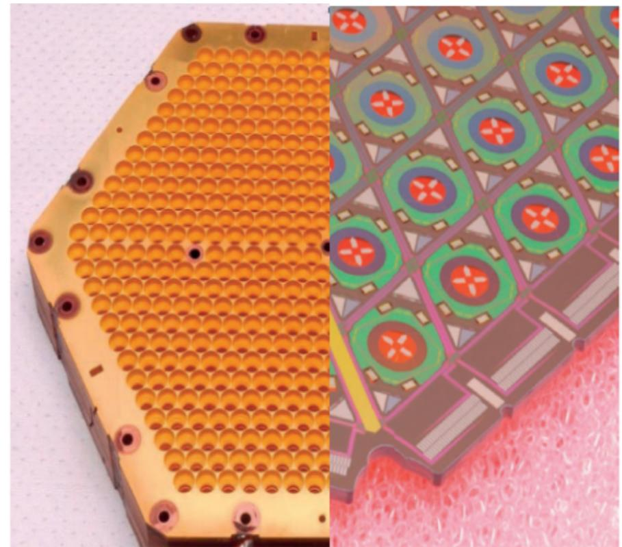
**Spline feed horns coupled to OMT detectors (NIST)**
