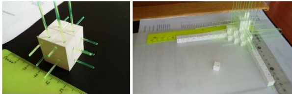
Figure 21: Schematic of the super-FGD structure.
