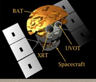
Swift/XRT (NASA) launched in 2004 3.5 m focal length, ~110 cm<sup>2</sup>@1.5 keV 0.2-10 keV Very versatile, adapted for fast ToO
