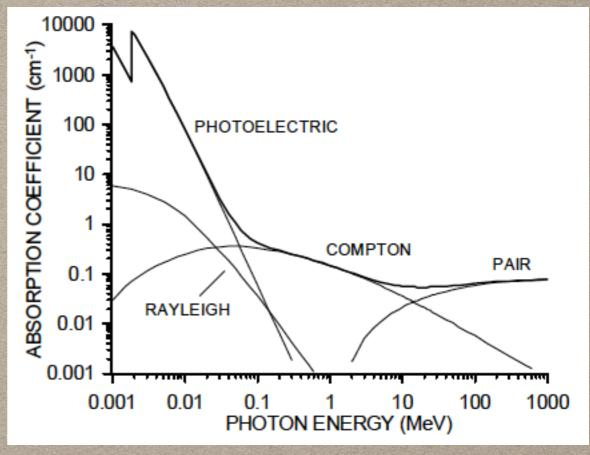
The probability of undergoing an interaction is an exponential function of distance. The fraction of photons that suffered any interaction after traversing a distance x is f=1-exp(- $\mu$ x), where  $\mu$  is the total absorption coefficient expressed in cm<sup>-2</sup>. *Photoelectric Absorption*
