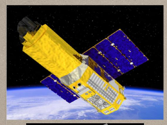
Suzaku (JAXA) 2005-2015 7.3 m focal length, ~400 cm<sup>2</sup>@1.5 keV Micro-calorimeter (failed soon after launch, cooling) Non-imaging Hard X-ray detector
