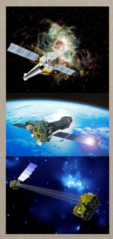
Chandra X-ray Observatory launched in 1999 by NASA 10 m focal length, 0.1-10 keV 600 cm<sup>2</sup> @ 1.5 keV, PSF: 0.5 arc sec
