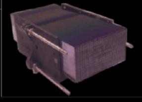
Silicon Pore Optics: 2 m<sup>2</sup> at 1 keV 5 arcsec HEW Focal length: 12 m Sensitivity: 3 10<sup>-17</sup> erg cm<sup>-2</sup> s<sup>-1</sup>
