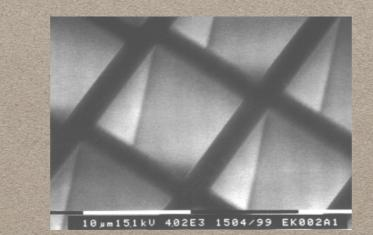
40 microns pitch lead glass plates produced by Photons
