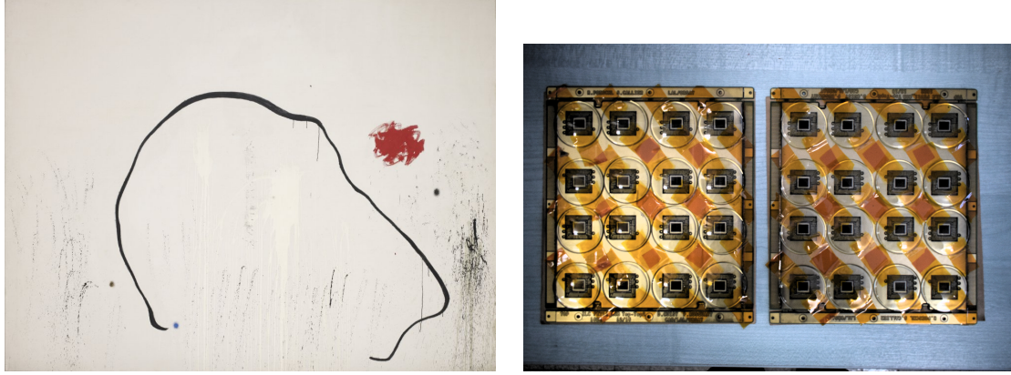
Figure 4. Left Temporary picture: La Esperanza del Condenado, J. Miró: Open single SLAB with FEV11 ASU, 16 SKIROC, interface card and DIF visibles. The silicon sensors are glued to the PCB in the other side. Right: two FEV11_COB boards with 16 SKIROC2a wire bonded. The ASICs are protected with watch glasses.
