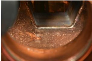
RFQ structures are affected by beam sputtering and surface degradation.
