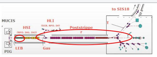
During accelerator commissioning in Summer it turned out that the RFQ can run only up to 6 V RF amplitude instead of 10 V!
