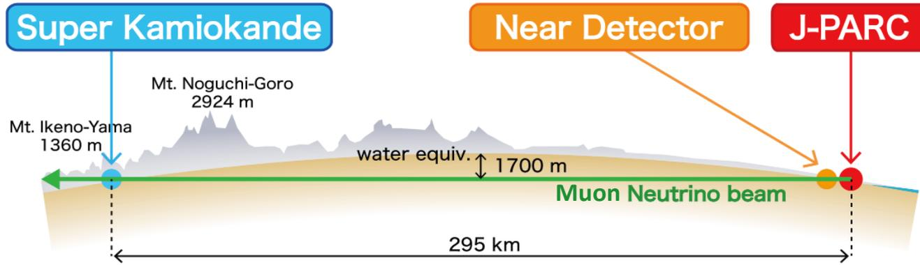
Use off-axis beam to give a narrow neutrino energy spread
